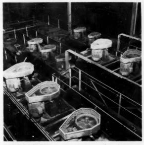
FLOTATION CIRCUIT now incorporates rougher, cleaner, recleaner, and scavenger stages with gravity flow of froth between stages.
